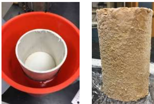
Figure 2. (a) Soil sample submerged in GWSs; (b) frozen soil sample.
